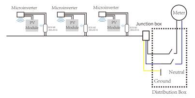
**WARNING:** Wiring colour code can be different according local regulation, check all the wires of the installation before connecting to the AC cable to be sure they match. Wrong cabling can damage irreparably the microinverters, such an issue is not covered by the warranty.
