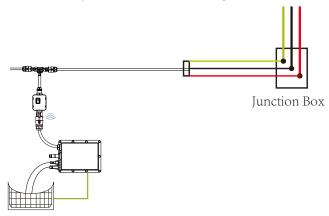
Step 5 - Connect Micro Inverter to the PV Modules
