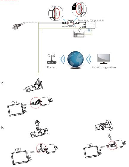
**NOTE:** For the connection between SUN-MI-Relay-01( Network and System Protection Dev -ice) and Micro Inverter, the tool(screwdriver) is needed.
