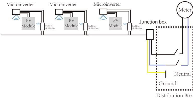
**WARNING:** Wiring colour code can be different according local regulation, check all the wires of the installation before connecting to the AC cable to be sure they match. Wrong cabling can damage irreparably the microinverters, such an issue is not covered by the warranty.
