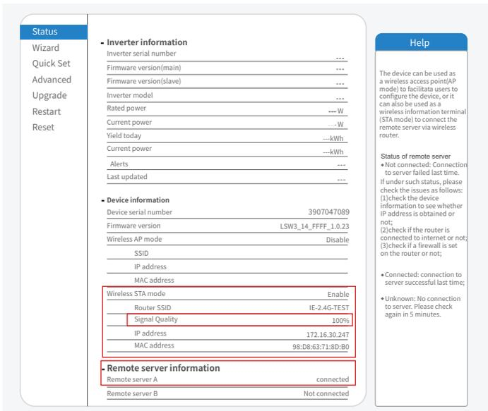
10. When it shows "connected" which means this Micro Inverter has connected solarman platform successfully. Generally speaking, it will be online after 10-15min after configuration successfully at the first time.
