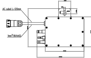
The AC wire on the micro inverter is a TC-ER wire with a wire cross-section area of  $1\text{mm}^2$ (18AWG).
