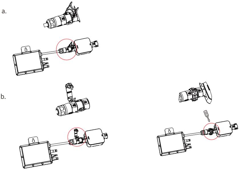
**NOTE:** For the connection between SUN-MI-Relay-01( Network and System Protection Device) and Micro Inverter, the tool(screwdriver) is needed.
