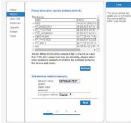
( Notice: If the signal strength (RSSI) of the selected network is <15%, which means unstable connection, please adjust the antenna of the router, or use a repeater to enhance the signal.
