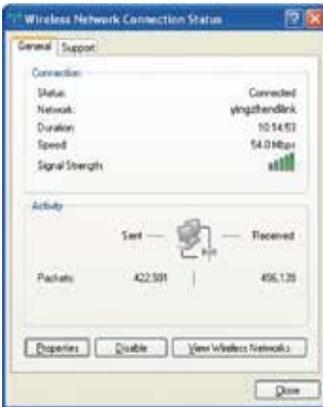
3.2 Select wireless network of the logger. The network name consists of AP and the serial number of the product. Input the password shown on the logger. Then click Connect.
