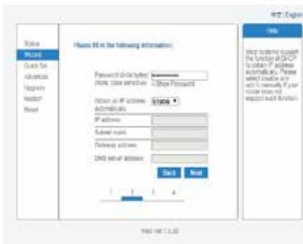
( Notice: Router password cannot be recognized if it contains any character such as '&', '#', '%', and blank space.
